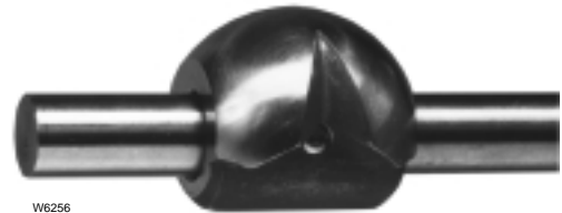
Micro-Notch V-Notch Ball for DN 25 or 1-Inch Valve. Use for C_v of 8.4 or Less
