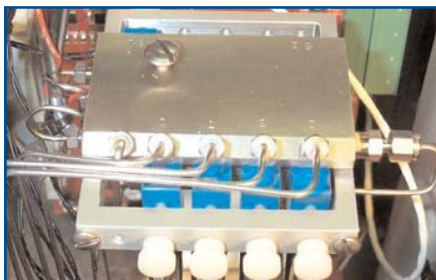
Internal heated four-stream switching module enables easy service and built-in expandability.
