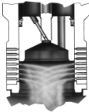
Cavitrol® Trim for Control of Liquid Cavitation
