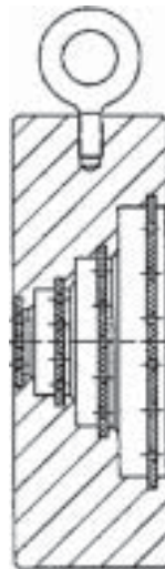
Four Stage Resistance Plate with Expanding Area Ratio
